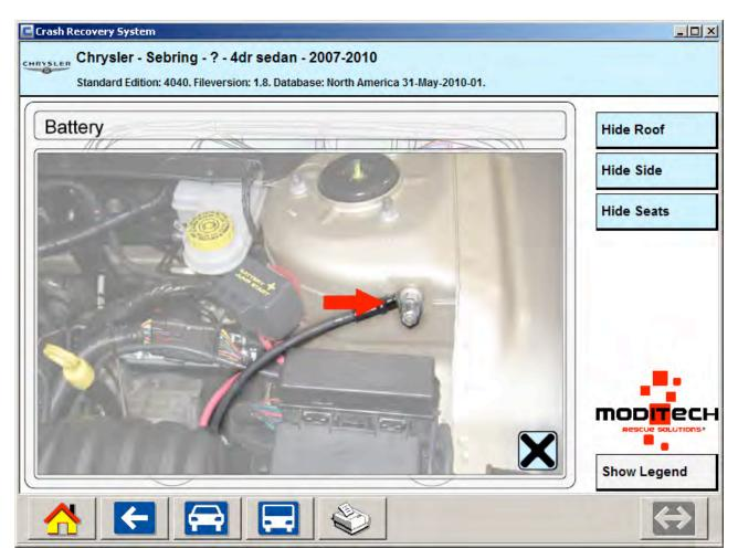
Furthermore CRS can guide you to the battery by giving information how to open the hood and trunk etc.
