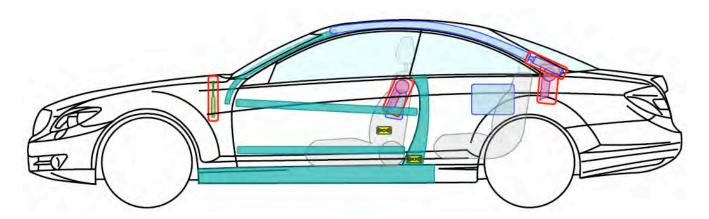
Mercedes-Benz CL. Reinforcement pipe in A-post. If you know where it is located, you can work around it or adapt your tactics (flap the roof to the front).
