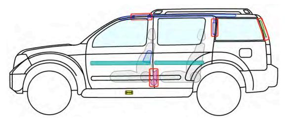
Looking at the side view of this Nissan Pathfinder the mounting positions of the inflators for the curtain airbags gets obvious. Cutting points can be selected with this knowledge. Removing the interior trim is not necessary anymore, however, it can be helpful in case the post have to be cut in close proximity to one of the mounting locations. Furthermore this schematic reveals that a seatbelt pretensioner is mounted at the base of the b-post and a pressurized strut is supporting the rear hatch.
