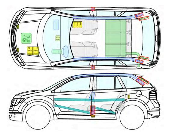
Ford Edge, Equipped with Frontal Airbags for the Driver and Passanger, Seat mounted side airbags and a curtain airbag on both sides of the vehicle and for all rows of seating. Addionally the airbag control unit can be found on the center tunnel of the vehicle under the dashboard.
