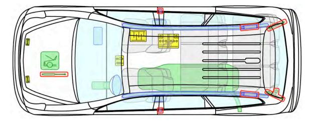
Performing electrical shutdown is much easier if the location of the battery is known. On this Chevrolet Traverse the battery is located below the passengers seat and can be accessed through an opening in the floor of the vehicle.
