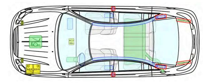
The battery of this Chrysler Sebring is located in the wheel well area of the vehicle. Even if you know where it is, it is very difficult to disconnect it. Additional information may be helpful. As you can see, the negative battery terminal can be disconnected from the body of the vehicle on the strut tower in the engine compartment.
