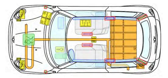
This Mini E carries a li-ion battery instead of the rear seats. The high voltage cabling running to the motor and to the charging point is also obvious. It's important to know where these components are to avoid damaging them.
