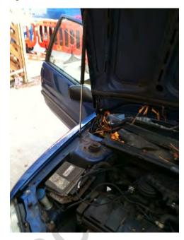
Another reason why we need to inspect where we are going to cut, as cutting through a pressurized strut can create a projectile that can cause serious injury. These also pose a hazard in car fires, and can become projectiles from out of the smoke, perhaps Breathing apparatus is not such a bad idea?
