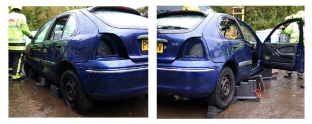
You can see in the above pictures the difference between the two types of equipment used with regards to trip hazards etc. Both sides stabilised ready for a dash roll. You can see on the right picture that there is also a risk that the rear door may come into contact with the rear step block, it would perhaps have been better placed at an angle, and this picture is just for training purposes.
