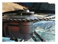
This is the Twin Saw, as you can see it is an electrically powered saw running on either 240v or 110v.
