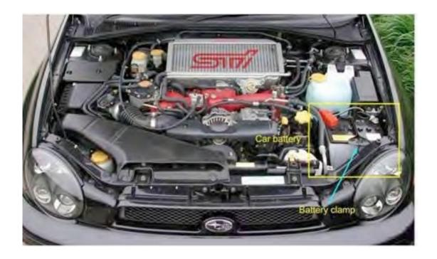
Batteries can be located in the engine compartment, under the drivers foot well, in the wheel arch and in the boot, these are the most common places to look however they may be in other locations.
